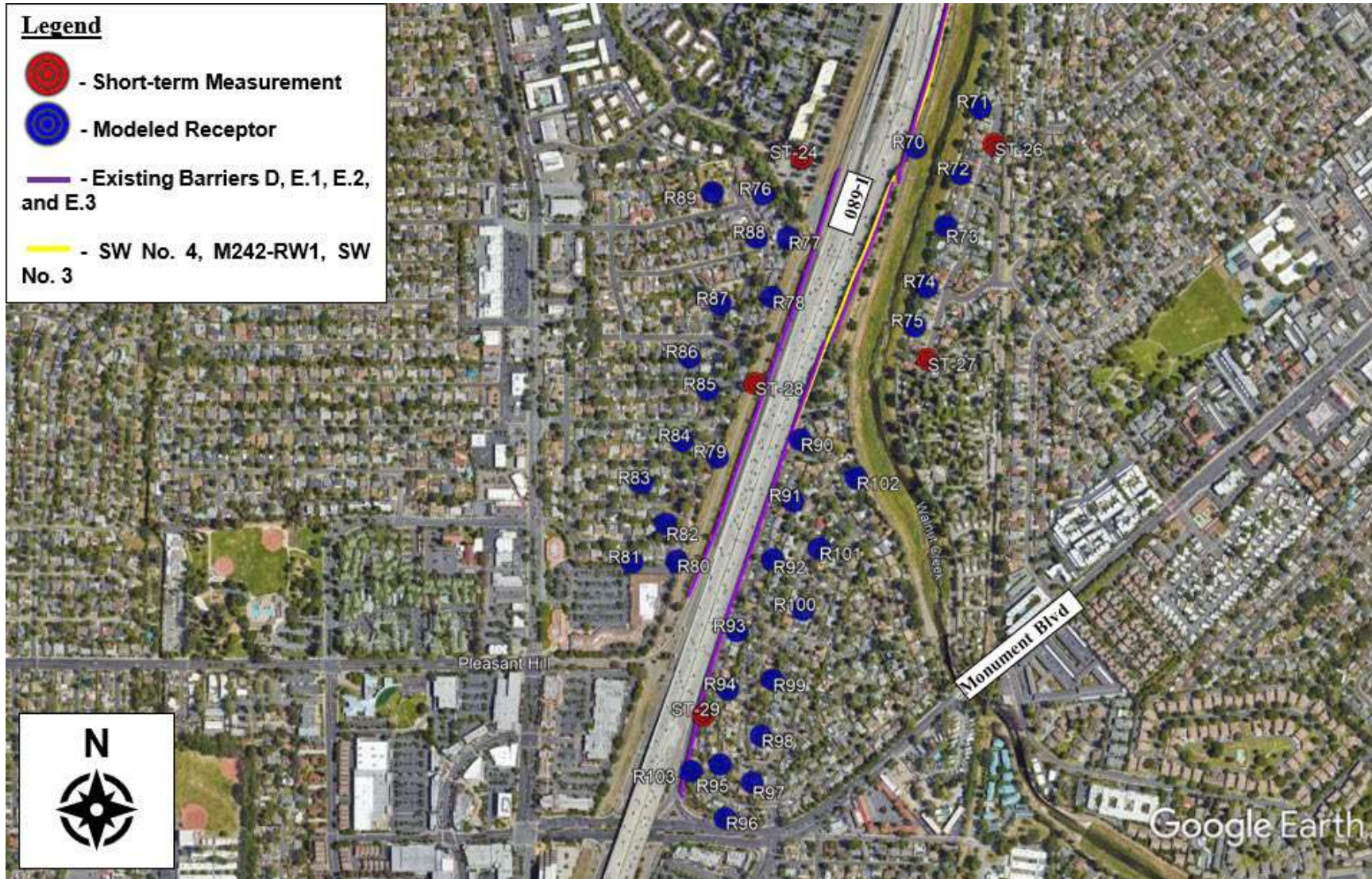
Figure J-5. Receptor Locations and Noise Barriers from south of State Route 242 to Monument Boulevard
