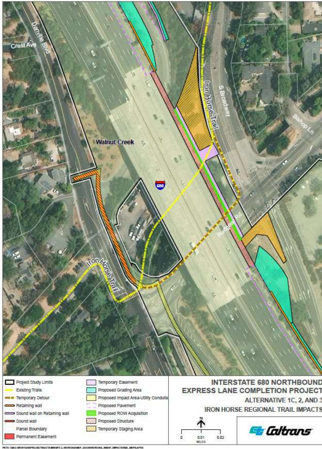
Figure 2.1.3-2. Alternatives 1C, 2, and 3: Iron Horse Regional Trail at Rudgear Road Undercrossing with Proposed Bridge Widening and Potential Temporary Trail Detour
