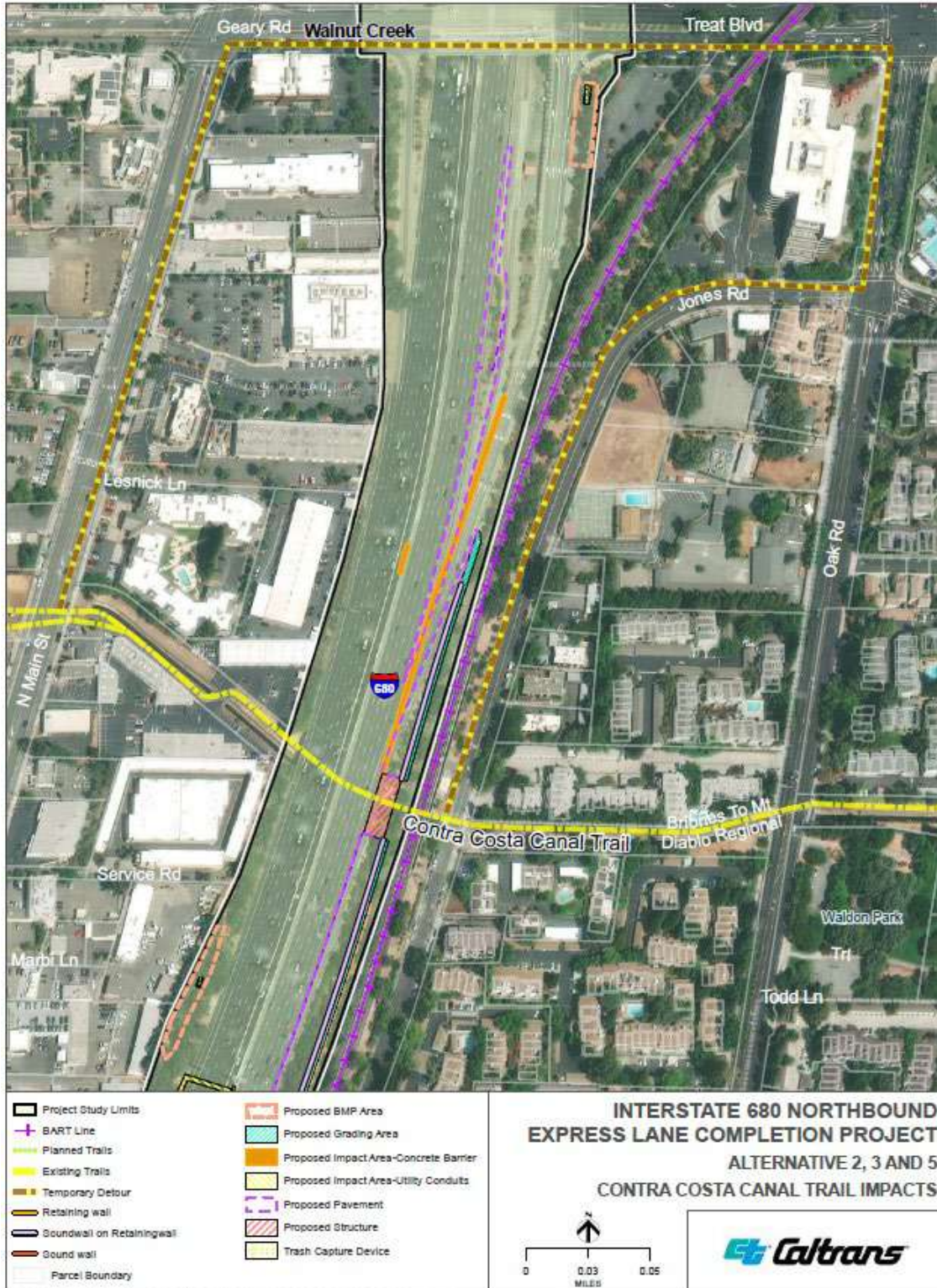
Figure 2.1.3-3. Alternatives 2, 3, and 5: Contra Costa Canal Trail at the Contra Costa Canal Undercrossing with Proposed Bridge Widening and Potential Temporary Trail Detour
