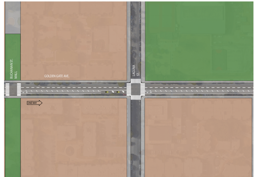
Figure 5-2: Plan View of Conceptual Golden Gate Avenue Road Diet Recommendation.
