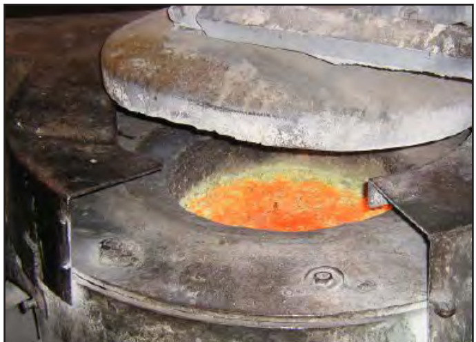
Bronze Kettle for Casting Spherical Bearing Components
