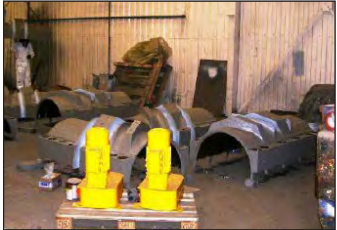
Cable Bands Ready for Painting
