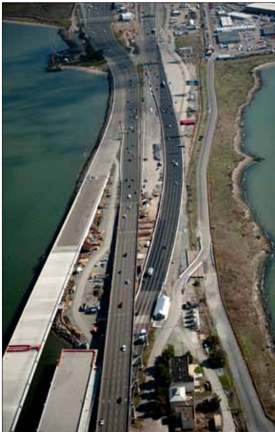
Aerial View of the Newly Opened Eastbound Oakland Detour with the EBMUD Outfall Crossing Structure on the right, the Relocated Clear Channel Sign and the Westbound Oakland Detour under Construction
