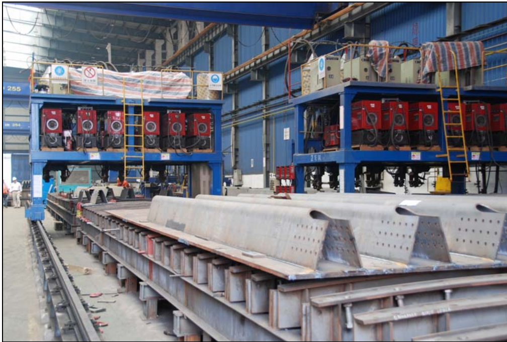
SAS - Deck Panel at the Zhenhua Port Machinery Company in China
