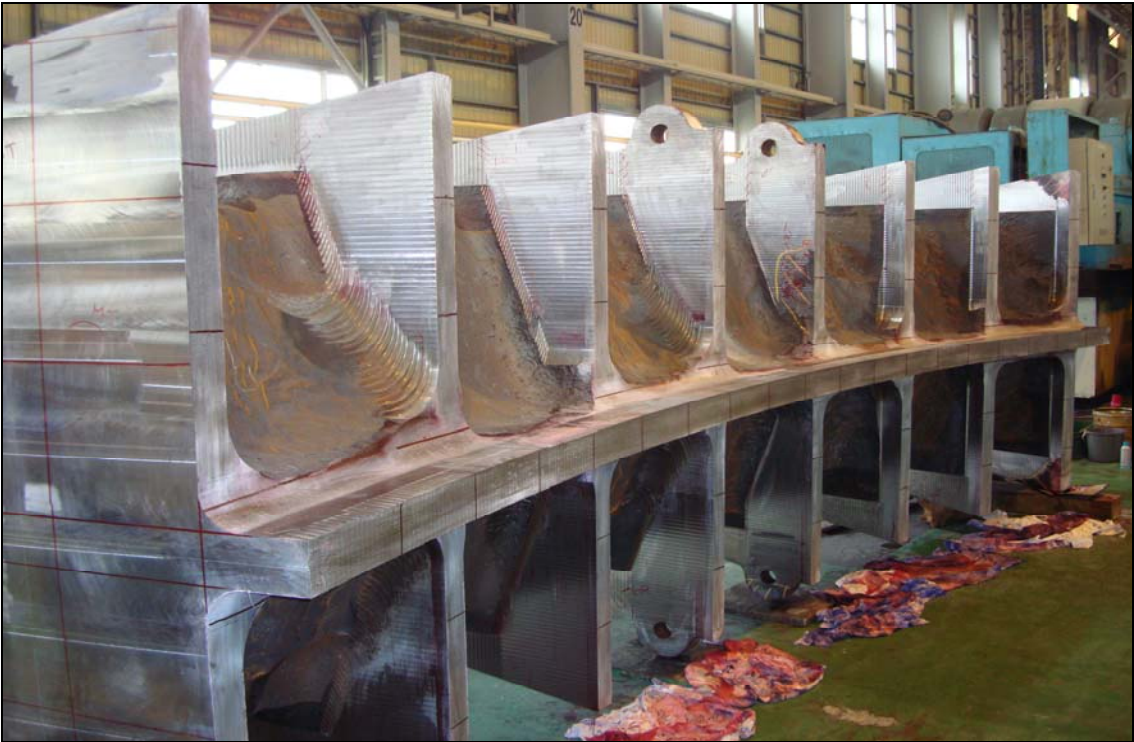
W2/E3 Saddle Fabrication during Ultrasonic Testing
