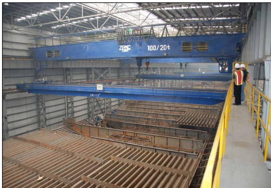
SAS - Deck Panel Fabrication
