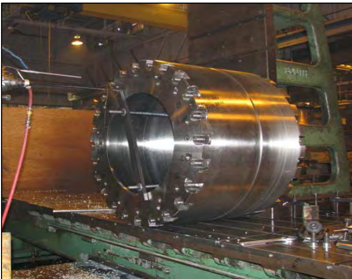
Stainless Steel Spherical Housing—Machining in the UK
