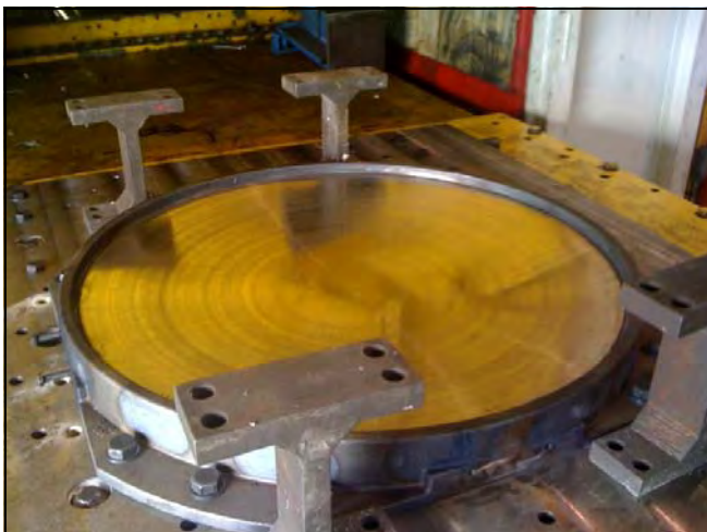
Prototype of Bearing for the Antioch Bridge Seismic Retrofit Project
