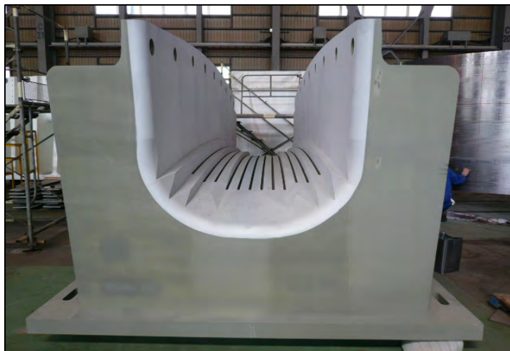
SAS East Saddle in Fabrication
