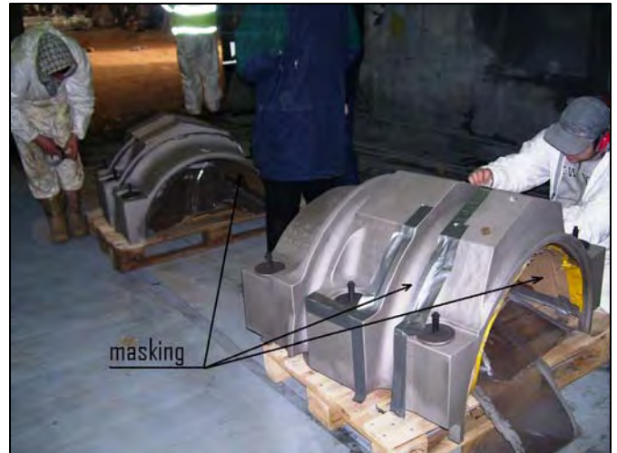
SAS Masking of Cable Bands Prior to Paint
