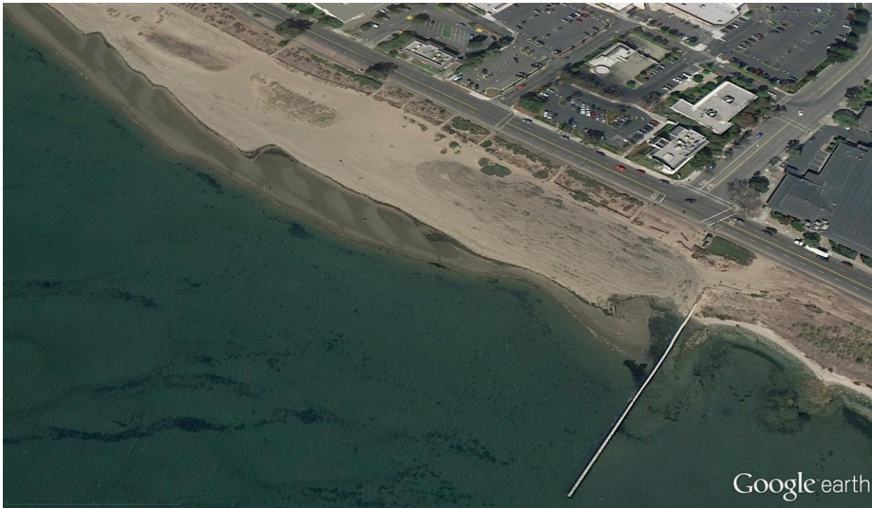
Figure 2.19 Beach – Robert Crown Memorial State Beach, Alameda (Beach Is Erosional and Maintained through Beach Nourishment [i.e., Imported Sand])
