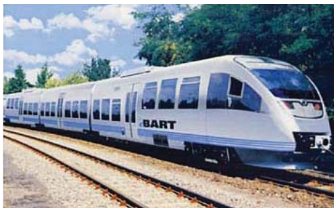
The eBART extension may use a train prototype like the Diesel Multiple Unit (DMU) car that can use existing tracks and rights-of-way.
