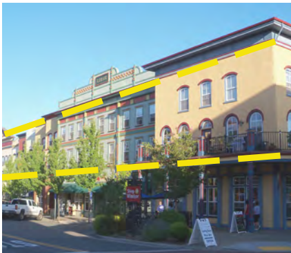
DG-18: These examples illustrate ways to express a base, middle, and top architecturally (top, bottom).
