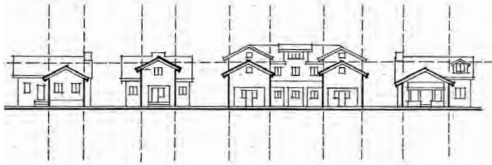
DG-55: This diagram illustrates how new construction can incorporate design elements of similar size, shape, and rhythm.
