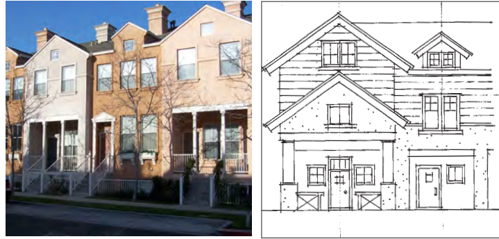
DG-59: Change in plane, porch design, window arrangements, and roof form create visual variety (left). Change in materials and subordinate volumes can help to break up a building's mass (right).
