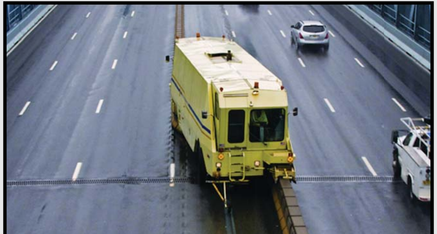
A moveable median creates a 4/3, 3/4 traffic pattern using 7 lanes
