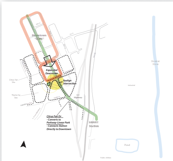
Realign the intersection of Cloverdale Blvd and Citrus Fair Dr Concept by Calvin Platt, Images by Rick Gosalvez
