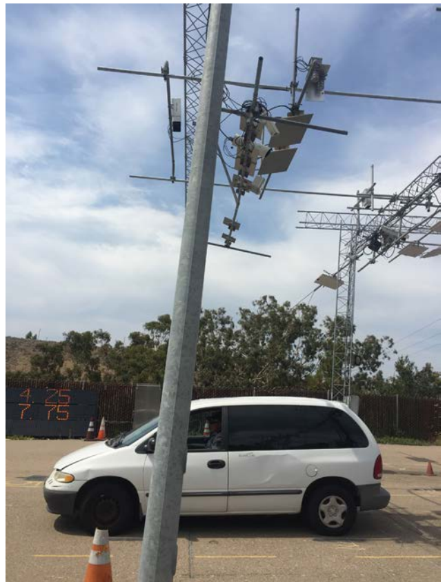
A test car goes through a test lane at the toll system factory acceptance test.
