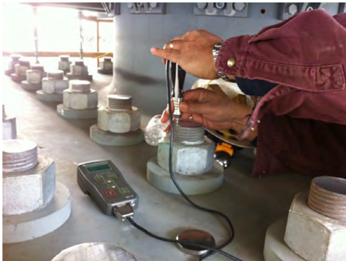
Figure 24 Photograph of Inspector Performing In-situ Hardness Test on Bearing Rod
