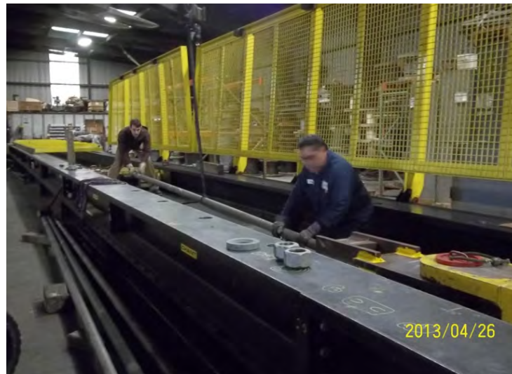
Figure 26 Photograph of Full-Sized Rod Being Placed into Test Rig
